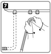
If you over stretch the pipe you can reduce the length by holding the pipe in two hands and slowly compress the corrugated folds using a gentle up and down movement.
