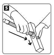
Place in the PRO-Fit pipe stretching tool.
